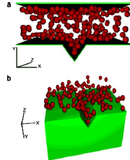
Geometry of the system used in the molecular dynamics (MD) simulations.
